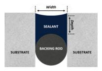
Wider joints can accommodate more total movement than narrow joints.
